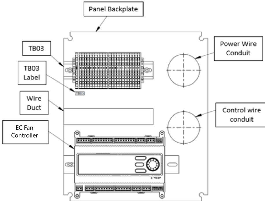
*Figure 4: Example Low Voltage Control Panel*
